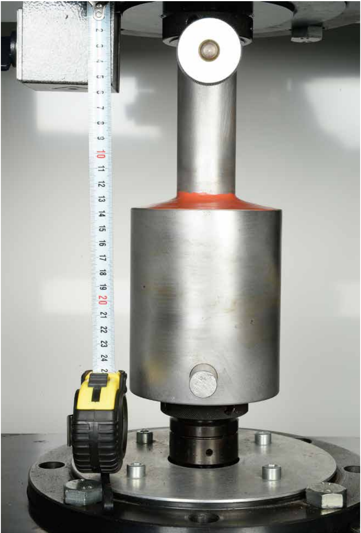
Test set-up for linear movement of the ducted pipe.
