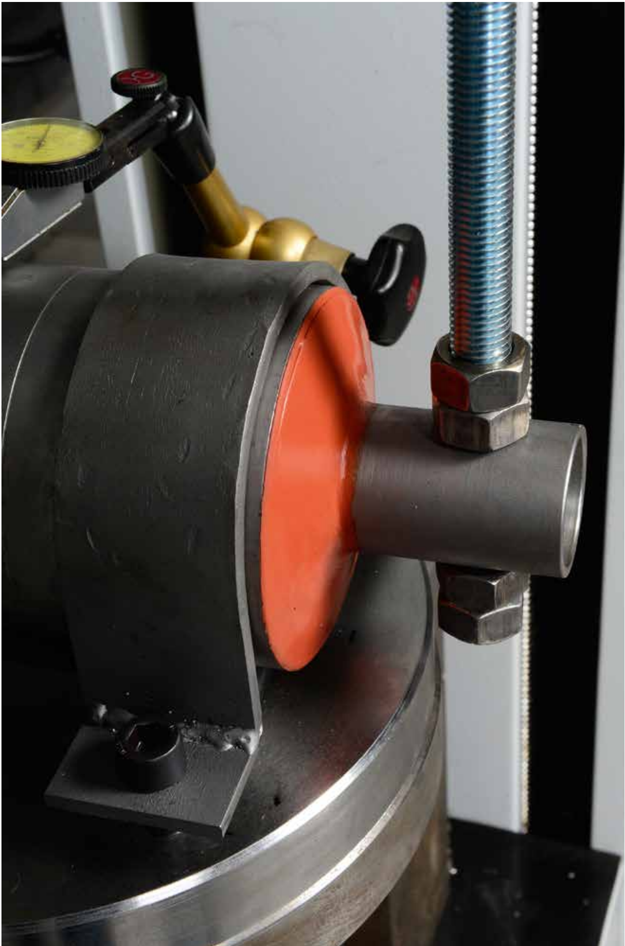
NOFIRNO sealing system with NOFIRNO filler sleeves around the ducted pipe and at both sides a layer of 20 mm NOFIRNO sealant.
